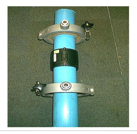
Suitable alignment clamps can assist with re-rounding of pipe
