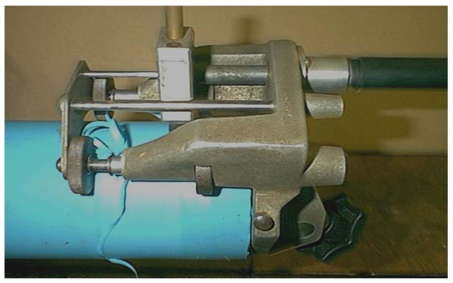
Mechanical scrapers provide a uniformed removal of between 0.2 to 0.4mm during pipe end preparation
