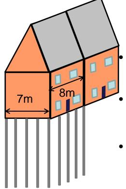
Roof with 40 ° pitch. South facing roof area of  $36m^2$
