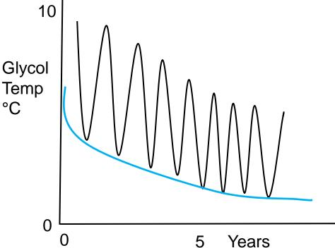
Heat pump efficiency and heat output is therefore lower than year 0.
