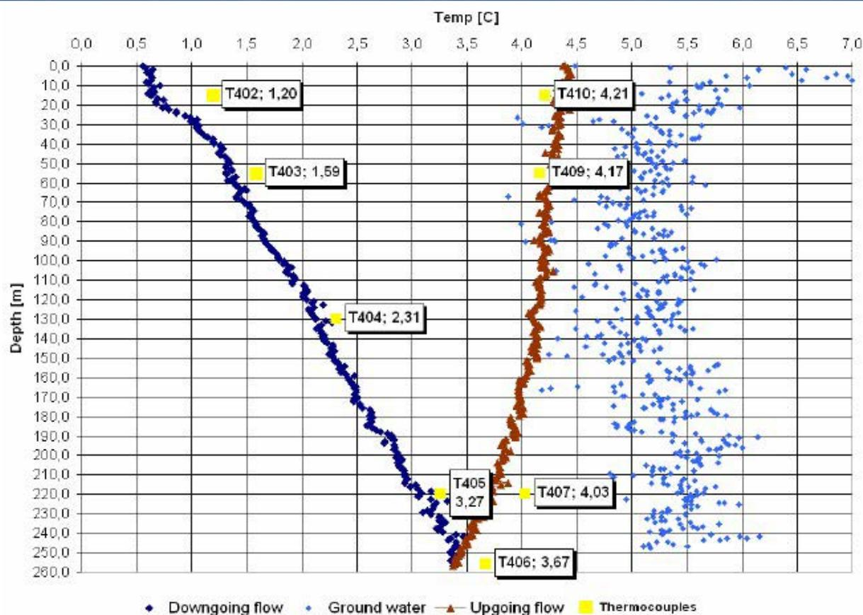
Figure 8: Average temperatures along the borehole during the first month of operation
