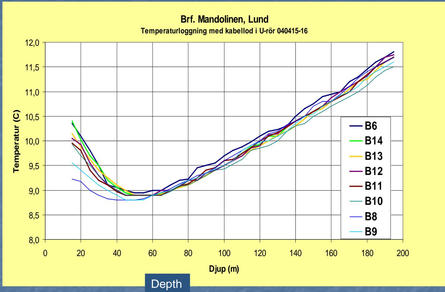
Temperature as function of borehole depth
