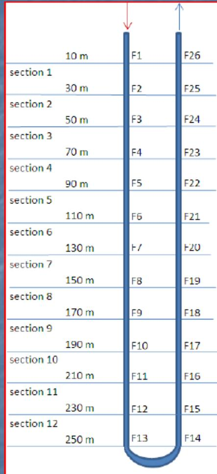
Measurement of heat balance in sections
