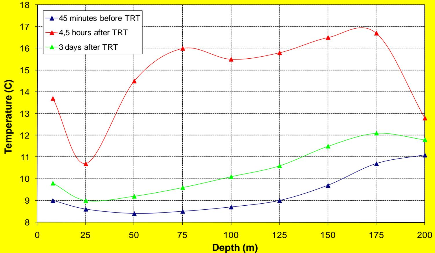
Temperature as function of borehole depth
