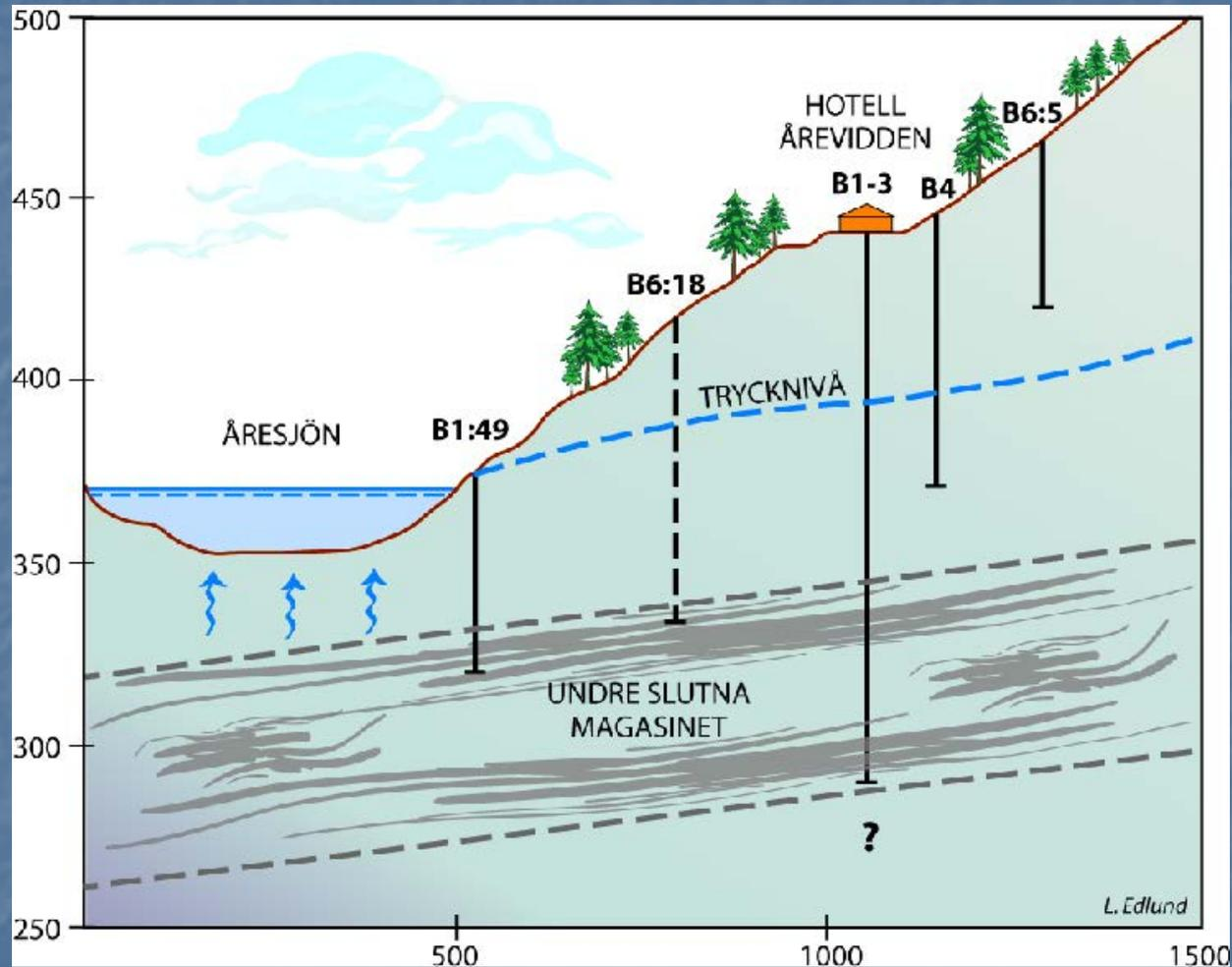
Groundwater flow between permeable layers with different hydrostatic pressure
