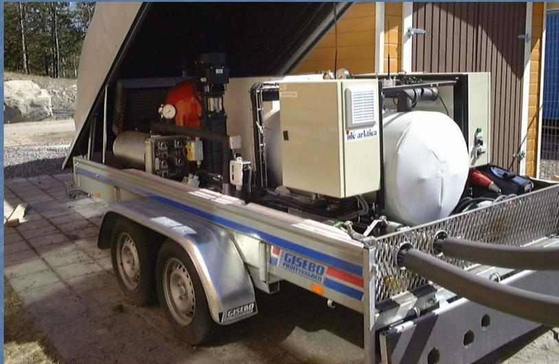
In 2004 a new TRT equipment was built at Luleå Technical University. It contains both an electric heater and a heat pump
