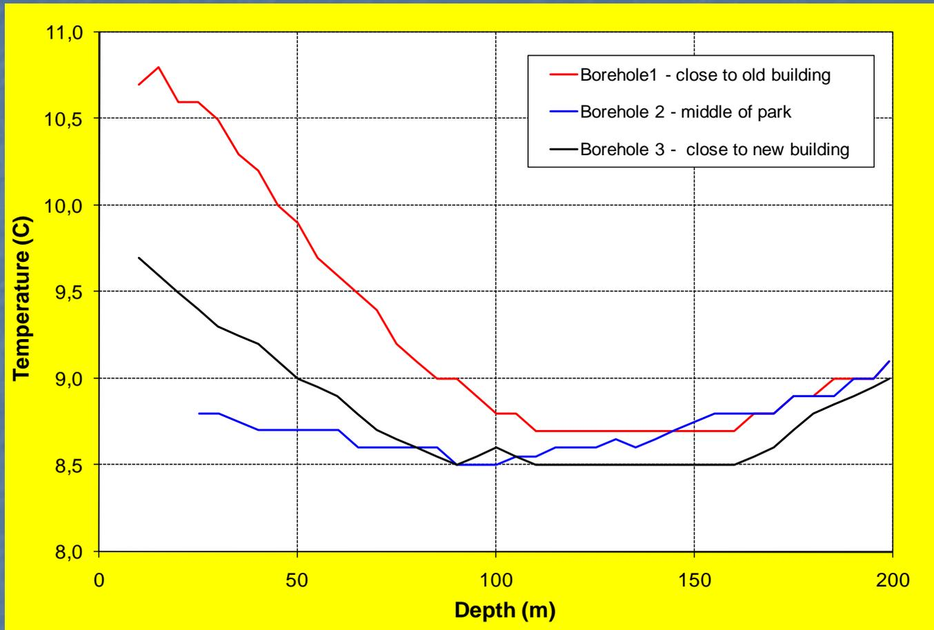
Temperature as function of borehole depth
