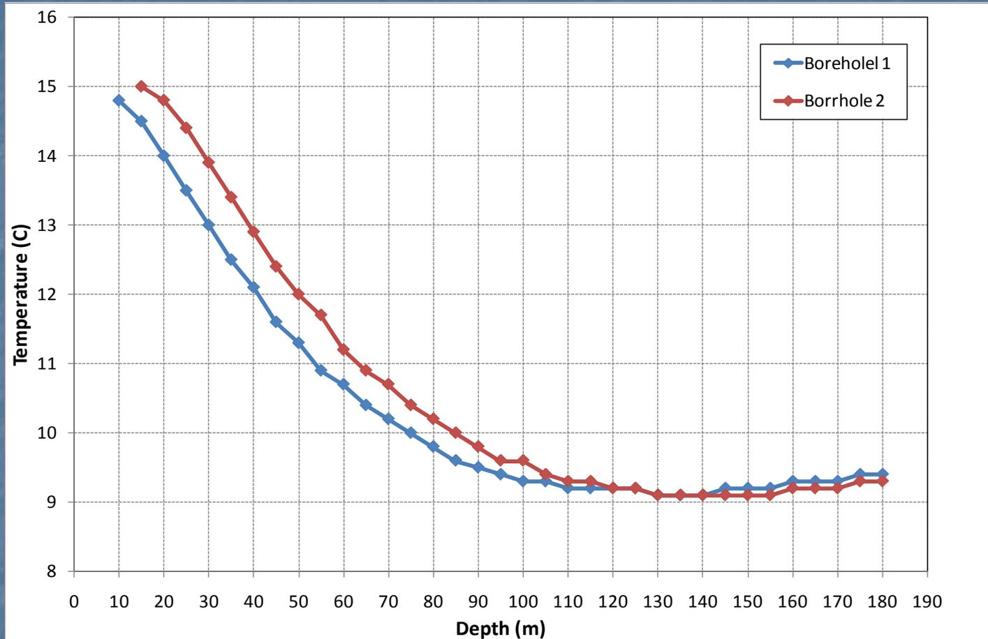
Temperature as function of borehole depth
