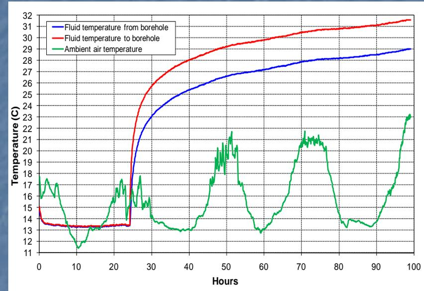
Measured injection rate, heat carrier fluid temperatures and ambient temperature
