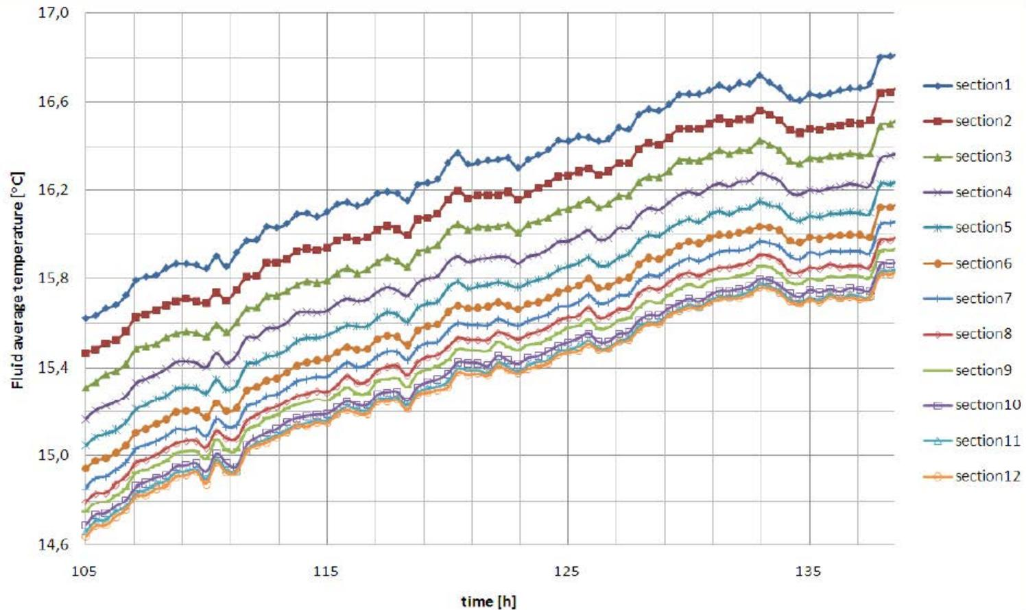
Fluid temperatures in each section during injection
