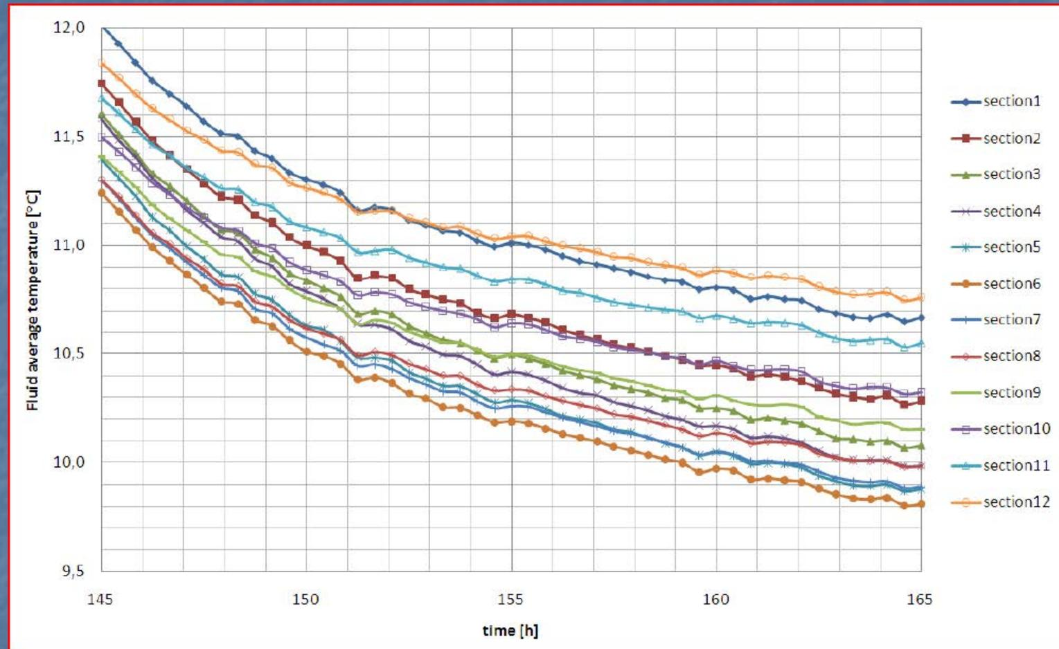
Fluid temperatures in each section during recovery
