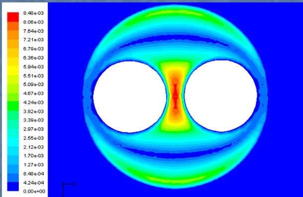
Single U-pipe in groundwater-filled borehole
