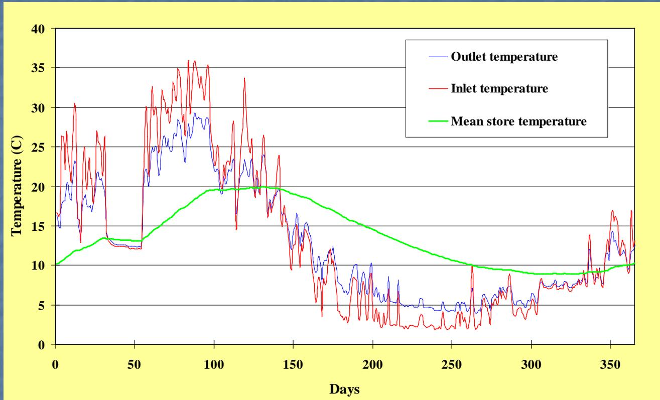
What is the relation between fluid temperatures and heat transfer rates for a specific borehole exchanger design?
