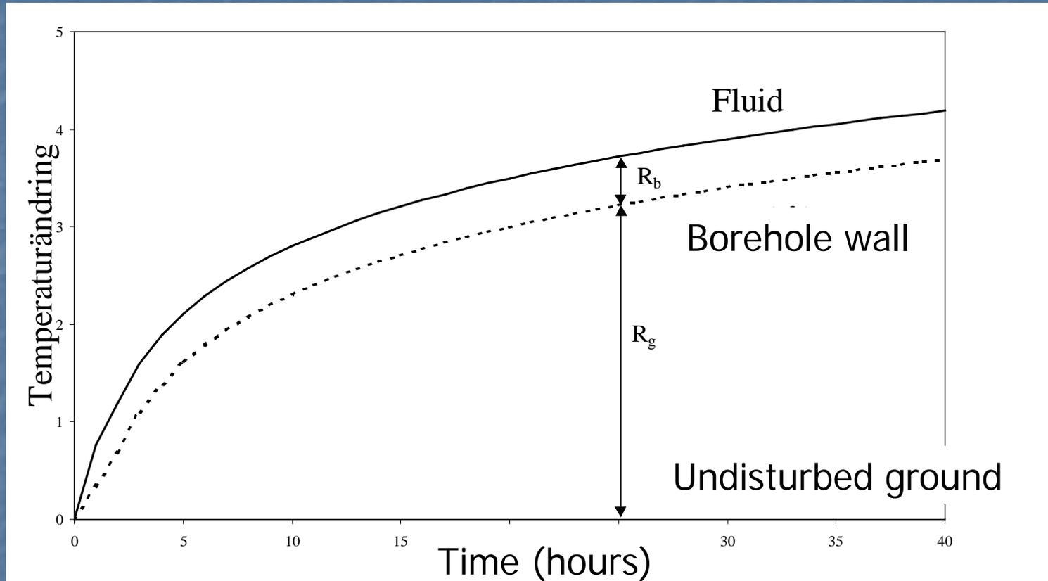
Temperature change when constant heat injection rate is supplied
