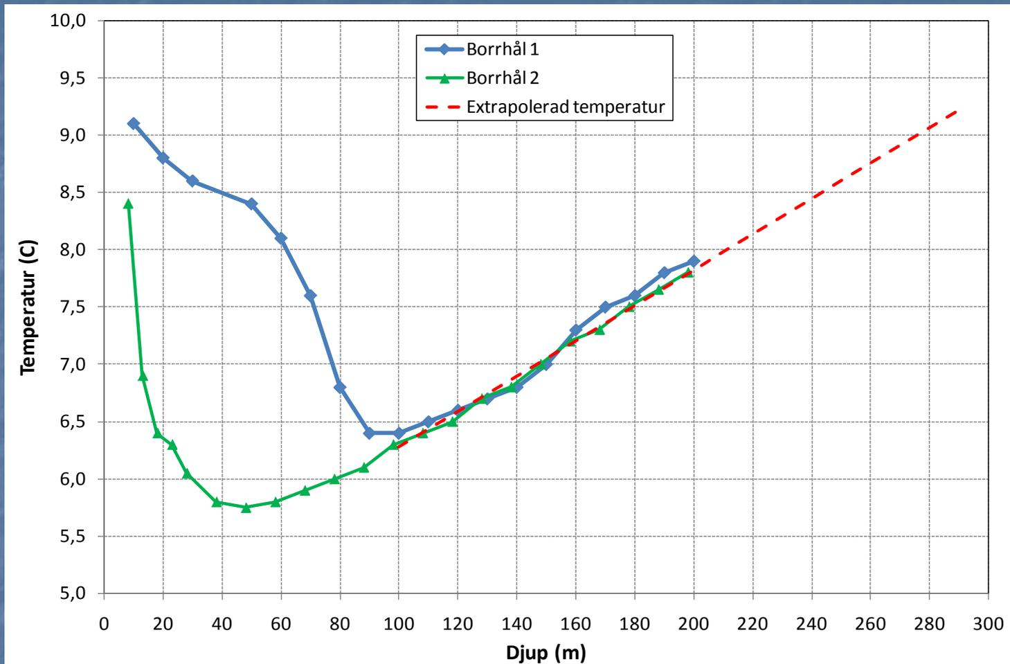
Borehole 1 disturbed by groundwater flow
