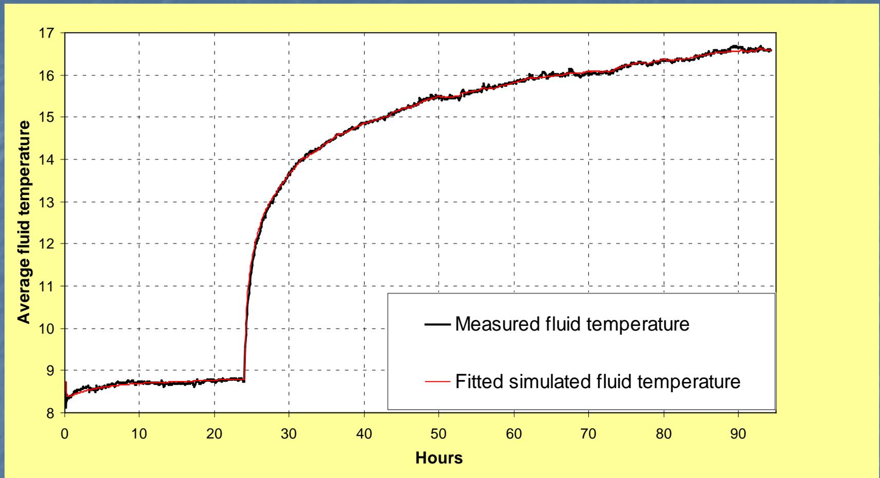
Fitting procedure of measured and calculated fluid temperatures gives effective ground thermal conductivity and borehole thermal resistance
