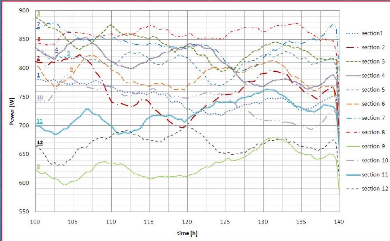
Power supplied in each section of the borehole
