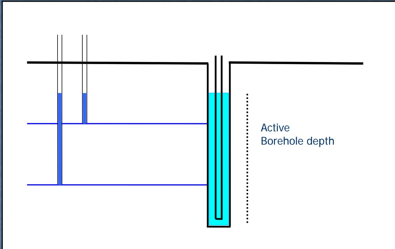
Groundwater-filled part of the borehole
