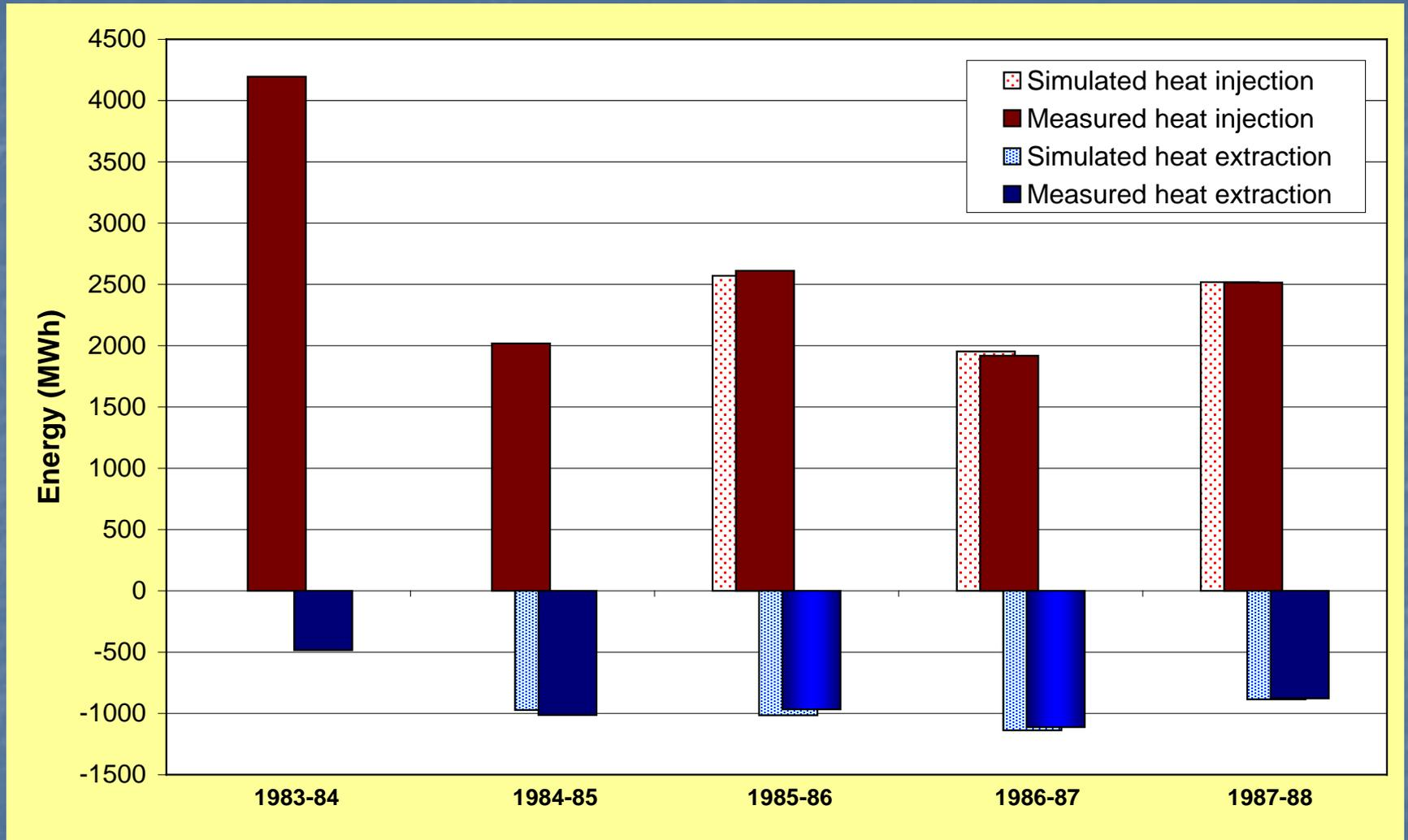
Measured and simulated energy balance 1983-1988
