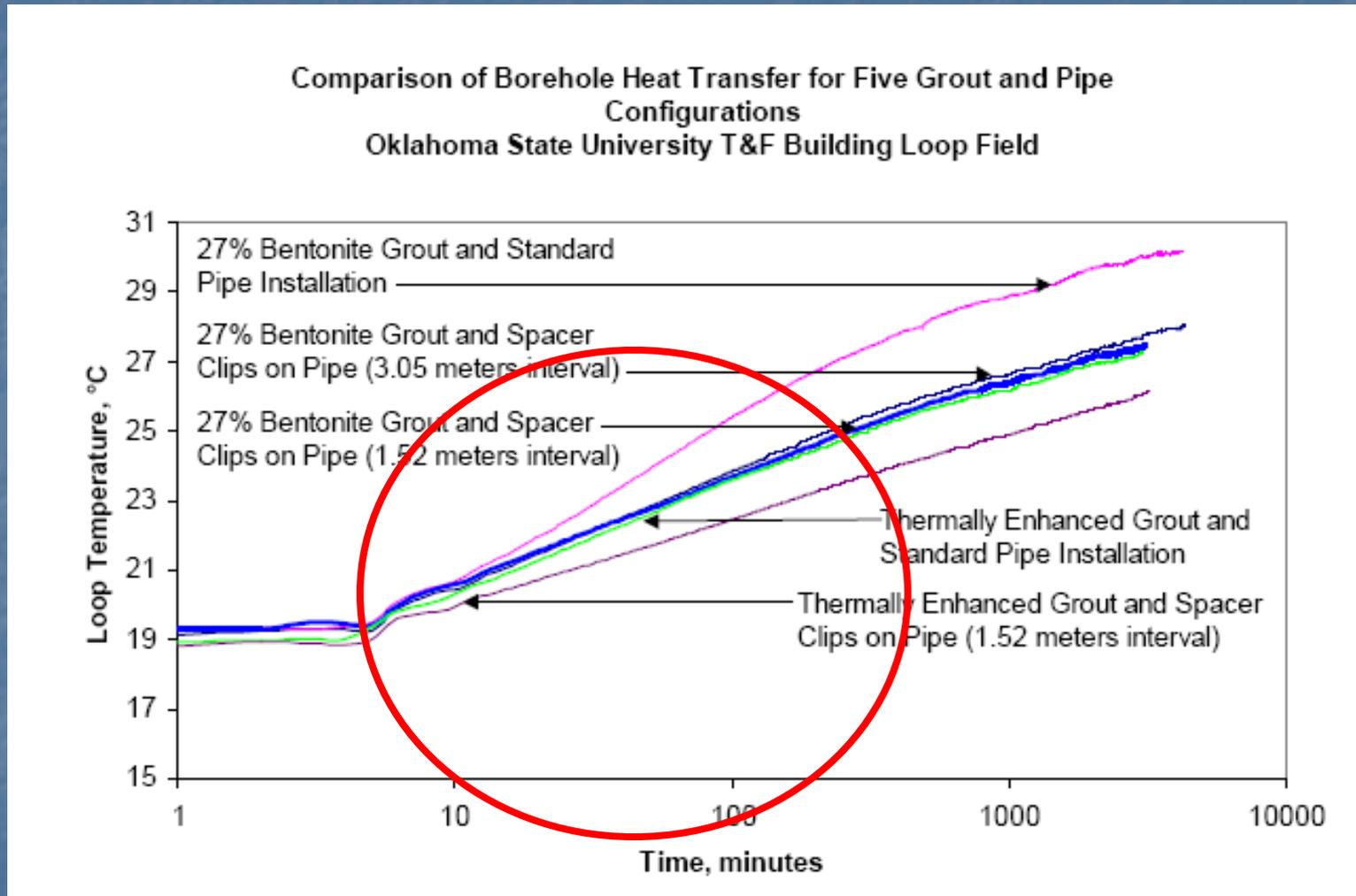
Fluid and grout thermal capacity
