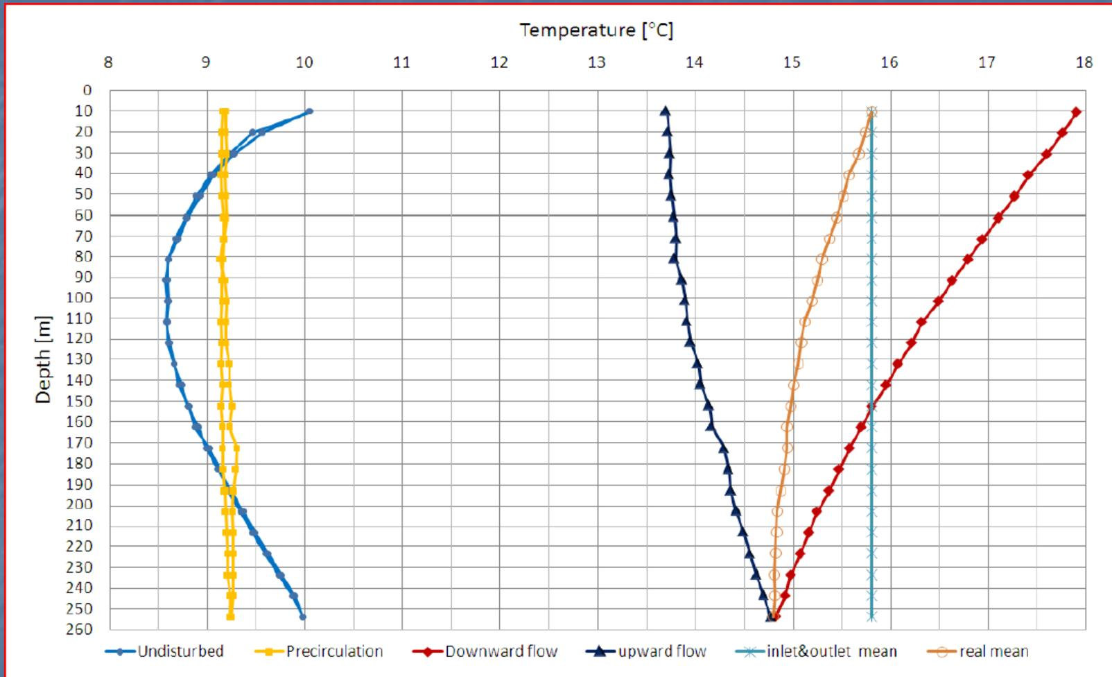
Vertical temperature profile before and during initial circulation of fluid
