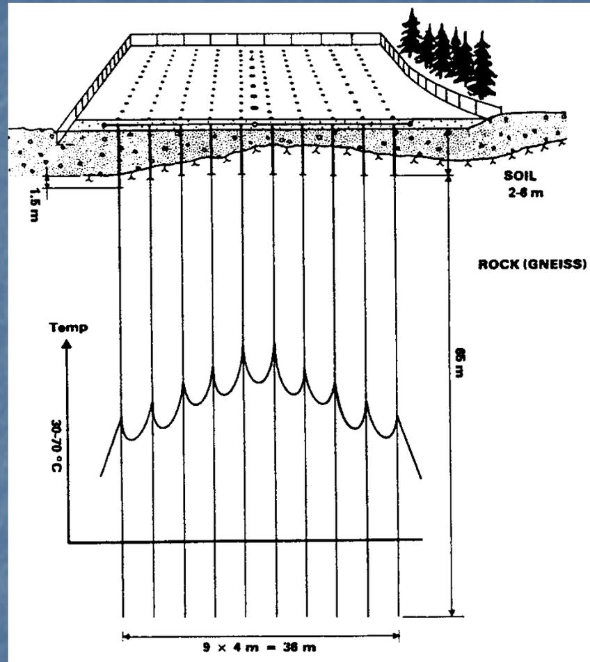
Borehole heat store: 120 boreholes depth 65 m
