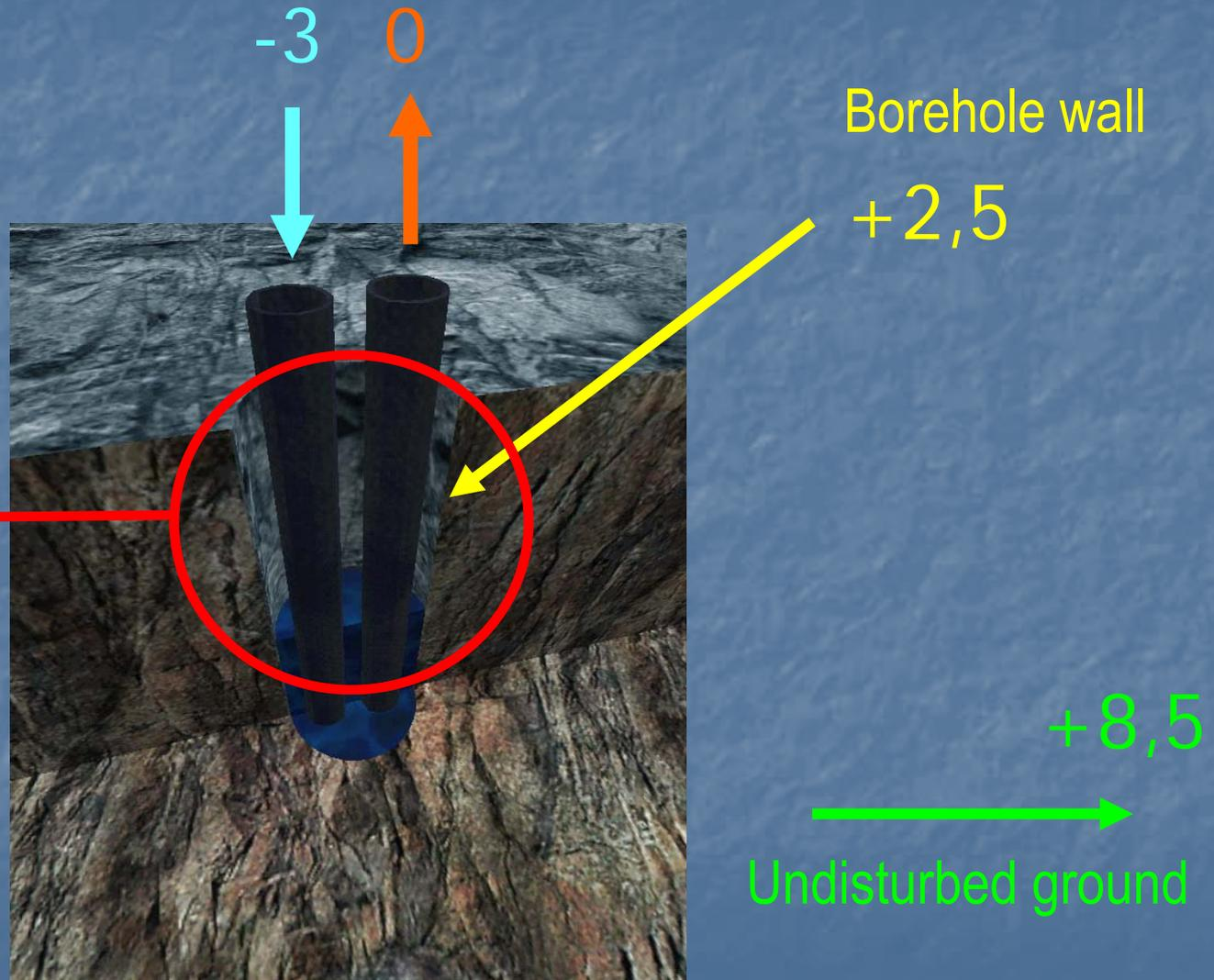
40 % of temperature difference between heat carrier fluid and surrounding ground within the borehole
