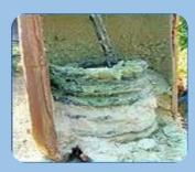
Scale blocks the pathways in heat exchangers and reduces the inner diameter of pipes and elbows, leading to restrictions in flow rate and pressure loss problems in systems.
