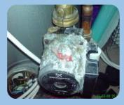
Scale often becomes encrusted on internal moving parts of pumps, valves, solenoids and other components, which leads to premature failures.
