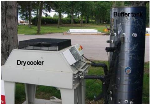
Rejected Heat via Dry cooler
