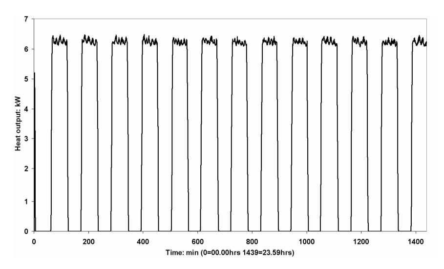
Typical heat pump loading of 50% for a day in November = 78kWh/ day
