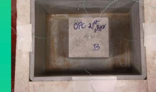
Readings stopped once cube temperature same as water temperature
