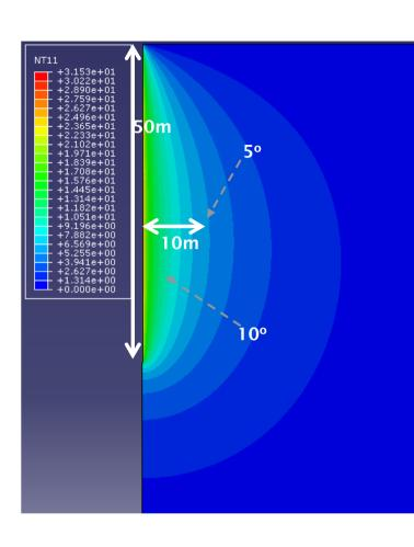
50m deep, 100mm borehole q=94W/m  $\lambda$ =3W/mK a=1.5e10-6m/s<sup>2</sup>
