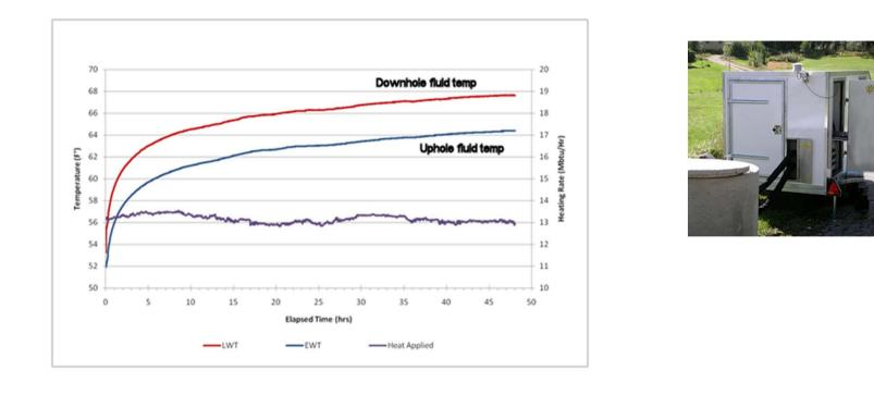
Advantage the in-situ thermal conductivity for the rock mass over the length of the borehole is measured
