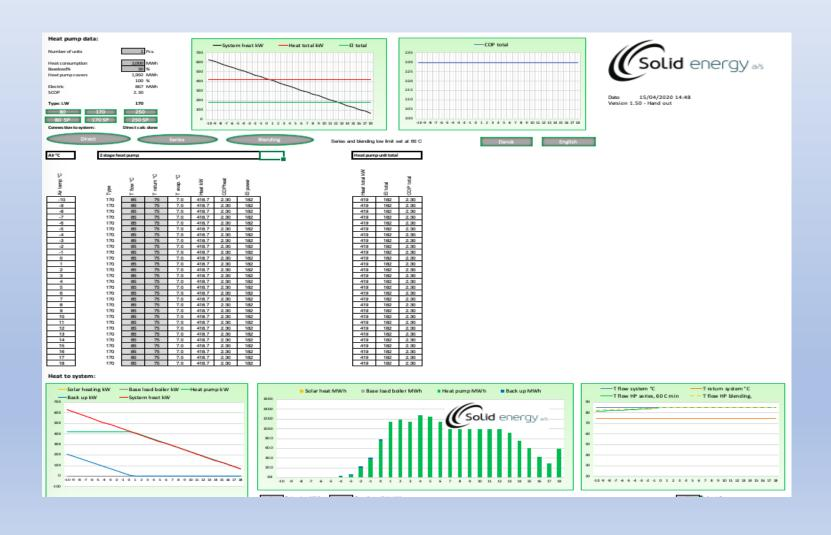
We have fixed the heat pump as a LW170 (nominal output 500kW) with the water source temperature at 10°C. We have varied only the flow and return temperatures to demonstrate the impact on the COP and similar scenarios with water source at 20°C (mine water?)
